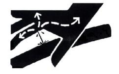
When disconnecting hydraulic lines, shut off hydraulic supply and relieve all hydraulic pressure.
