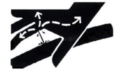
When disconnecting hydraulic lines, shut off hydraulic supply and relieve all hydraulic pressure.
